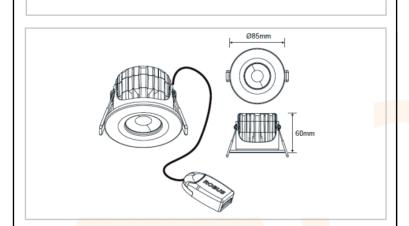
**LED** Cap Type **Total Power (W)** 4.7 Lumens (Im) 410 **Beam Angle** 60 Lamp Life (Hrs) 30000 Number of LEDs 6 (6S1P) Comparable To 50W halogen **CRI** CCT (K) 3000 Efficacy (Im/cctW) 87 Lux at 1m 390 **Power Factor** 0.9 Colour White Cut Out (mm) 72 Projection (mm) Recess Depth (mm) 55
