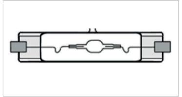
**Technical Specification** 12500 Lumens Power (W) 141 LPW 89 CCT 4200 >90 CRI 96 Lamp Volts 1.8 Lamp Current (A) Nominal Life (Hrs) 15000 RX7s Base Type 135 Max Length (mm) Diameter (mm) 23 +
