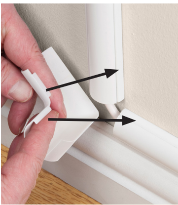
All Clip-Over accessories have grip tabs. The grip tab simply clips over the top of the length.
